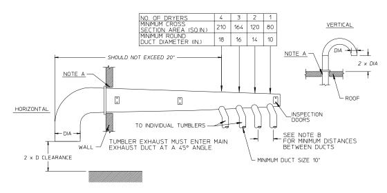
IMPORTANT: NO MORE THAN 4 DRYERS CAN BE CONNECTED TO ONE COMMON DUCT ( VENT ).
